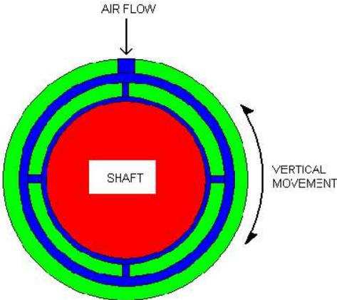
Fig. C: Round bearing-side view
